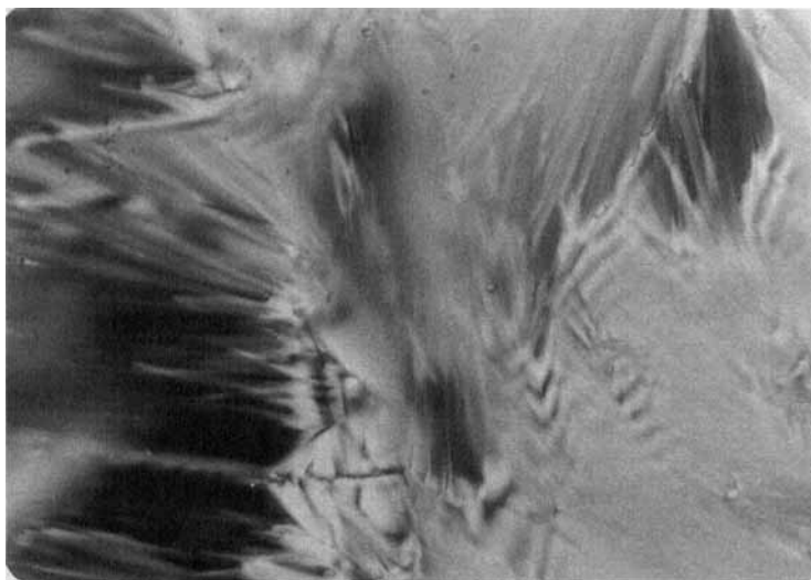
Figure 8. S_A , simple fan-shaped texture. Crossed polarizers, 112.9^\circ\text{C} , \times 400 , on heating 7\text{C} .
